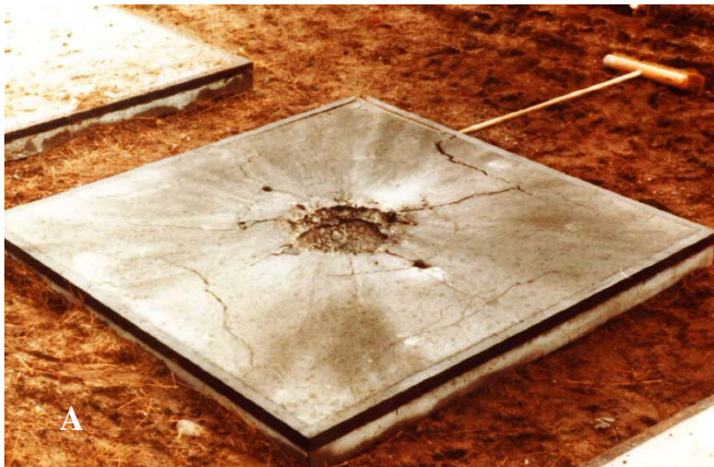
Figure 08: Impact tests Dutch Ministry of Defense. A is normal reinforced concrete, B is SFRHPC (Source: A.Verhagen - Breda).
