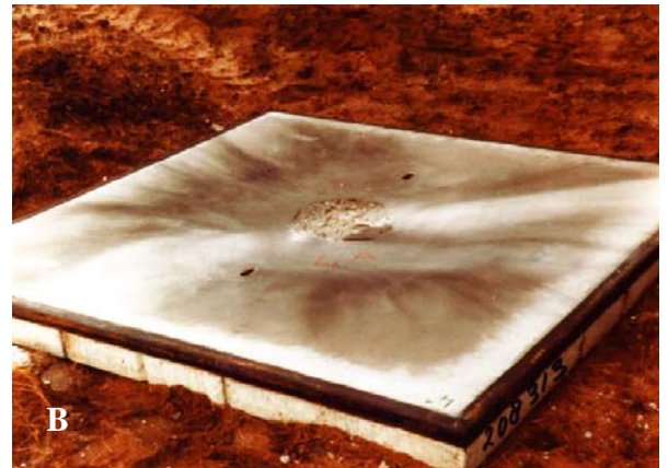
Figure 08: Impact tests Dutch Ministry of Defense. A is normal reinforced concrete, B is SFRHPC (Source: A.Verhagen - Breda).
